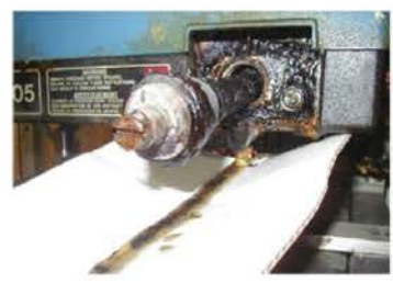
Joint Disrupted / Opened While Still a Hot Liquid
