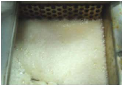
Foam in Hot Melt at Applicator
