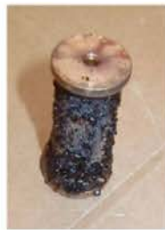
Oxidation, Charring of Hot Melt
