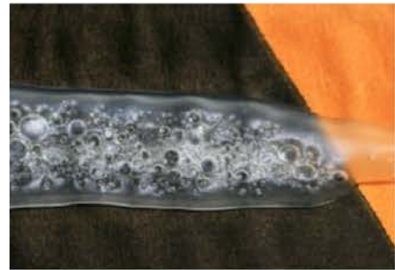
Bubbles in Hot Melt on Substrates
