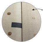
The board on the left absorbs water quickly, which indicates the adhesive most likely will have ideal bond strength. The board on the right doesn't absorb water as quickly and therefore the adhesive will have weaker fiber tear.
