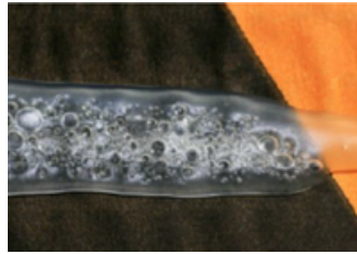
Bubbles in Hot Melt on Substrate
