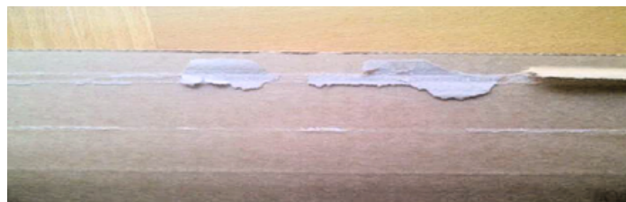
Bead width variation on substrate
